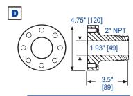
**NOTE:** The dimensions of the threaded neck on this adapter are equivalent to Schedule 80 pipe.
